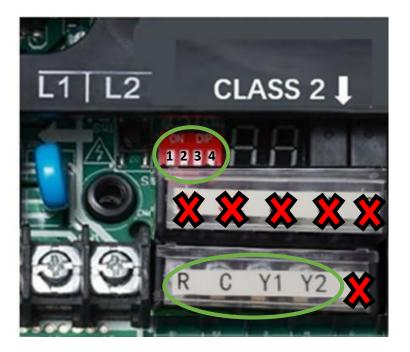
DIP switches must be changed while unit is powered off.
